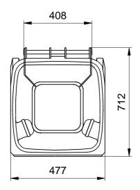
Mobile Waste Containers MGB 180 Litre Sizes, Measures, Dimensions: Hight 1063 mm; Width 477 mm; Depths 712 mm
